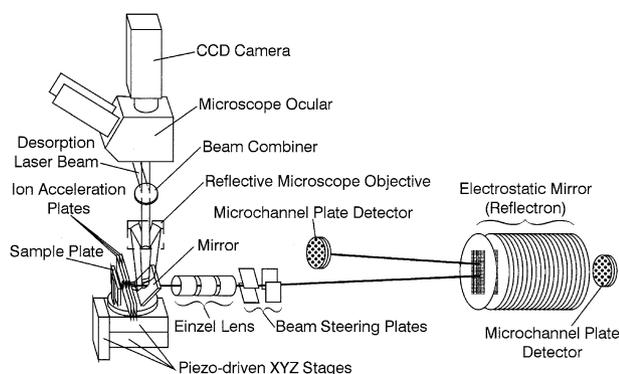
**Figure 1.** Schematic of the microscope-laser desorption/ionization-reflectron time-of-flight mass spectrometer.
