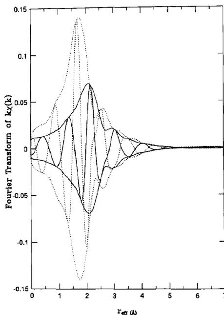
Fig. 5. Decomposition of the fit. The dotted line is the calculated EXAFS signal resulting from the first carbon shell and the solid line is the calculated EXAFS signal resulting from the second carbon shell.
