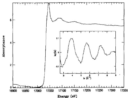
Fig. 2. Raw absorption data at 10 K in energy space. Inset: corresponding  $k$ -space transform of the same data.
