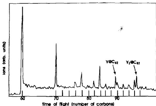
Fig. 1. Laser desorption, laser ionization (193 nm) time of flight mass spectrum of the sample.
