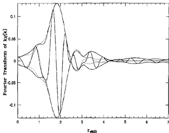
Fig. 4.  $R$  space data (solid line) and a fit to the data with an assumed endohedral geometry (dotted line). The fit was calculated with only the first two carbon shells.
